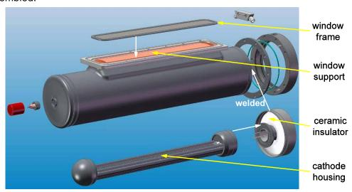
When an emitter eventually fails, the user will replace it with a spare and send the used one back to the supplier. At the supplier, the window frame is milled out and the tube is cut open. All parts are cleaned and possibly replaced (e.g. the filament wire). The tube is then welded together again and a new window frame (with the critical titanium foil) is welded in.
